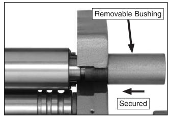
Figure 33. Securing top roller (T21324 shown).
